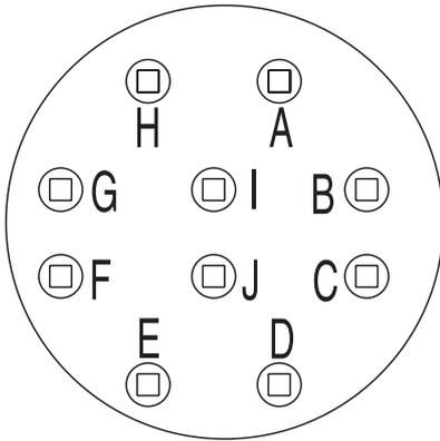
Put the knob on RC1 at minimum/max, put one ohmmeter from pin A - B and measure the resistance.
