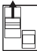
In case of intervention by this protection device, reset the G.F.I. switch by moving the lever to the ON position. In case of another intervention, verify that there are no faults in the tools connected, or replace the G.F.I. switch with another one of matching specifications and/or contact the Service Department.
