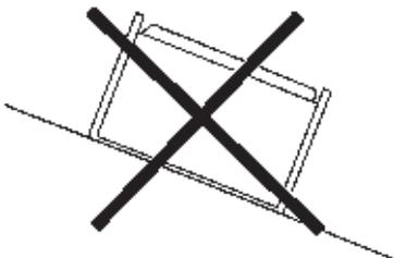
Maximum leaning of the machine (in case of dislevel)
