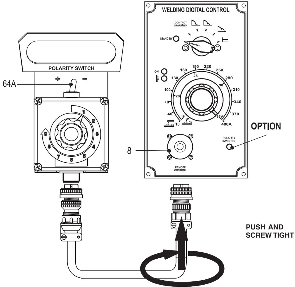
Is it possible to connect the RC1, to all **DSP** engine driven welders.
